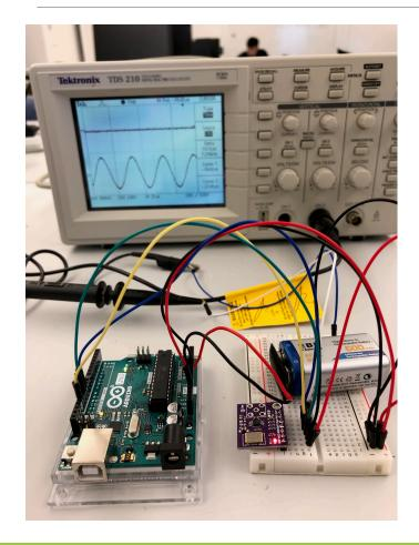
Function generator chip and Arduino microcontroller communicating
